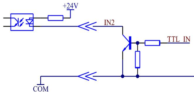
Figure 3-5 Input: External Logic Level Connection Diagram
