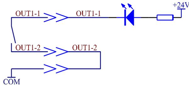
Figure 3-2 Output: The Internal Power Connected with Indicator Light
