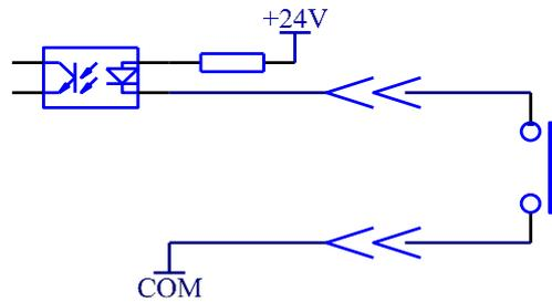
Figure 3-3 Input: External Switch Connection Diagram
