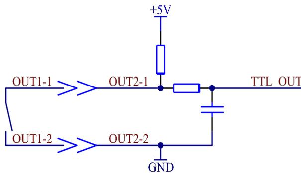
Figure 3-4 Output: External 5V Power Supply to Level
