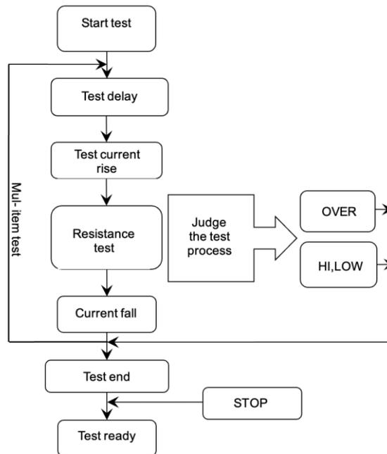
Figure 3-1 Block Flow Diagram of the Instrument
